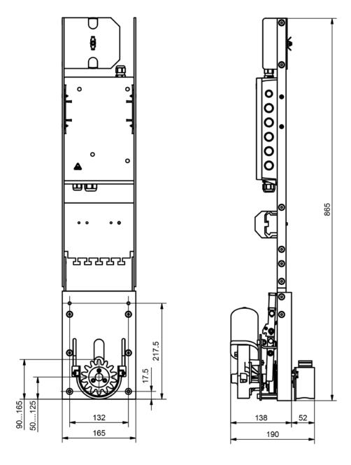
① Dimensions are stated in millimeters. Drawing shows the version ORBIT 800A. You will find the drawings of the versions ORBIT 800A-L and ORBIT 800A-S in our installation and operating instructions.
