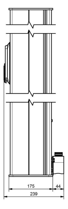
① Dimensions are stated in millimeters. Drawing shows the version ORBIT 800. You will find the drawings of the versions ORBIT 800-L and ORBIT 800-S in our installation and operating instructions.
