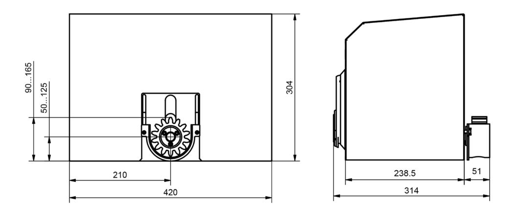
① Dimensions are stated in millimeters. Drawing shows the version NOVA 800. You will find the drawings of the versions NOVA 800-L and NOVA 800-S in our installation and operating instructions.
